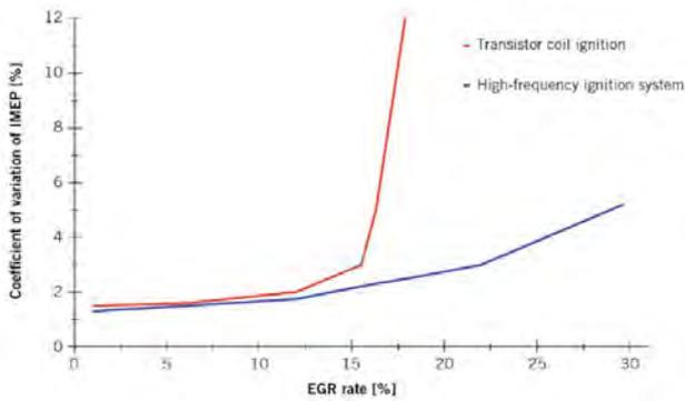
**Running smoothness comparison between a conventional 90 mJ transistor coil ignition (TCI) and the high-frequency ignition system (HFIS) EcoFlash in the case of progressive charge dilution by exhaust gas recirculation (operating point 2000 rpm and IMEP = 6 bar)**
