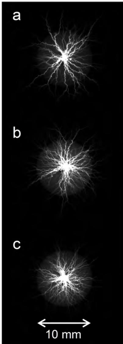
**Corona formation at high pressures in nitrogen; each individual image shows image sequences integrated over an ignition process with a duration of 500  $\mu$ s: 20 bars chamber pressure and 80 % DC power setpoint (top), 30 bar and 95 % (middle) and 40 bar and 100 % (bottom)**
