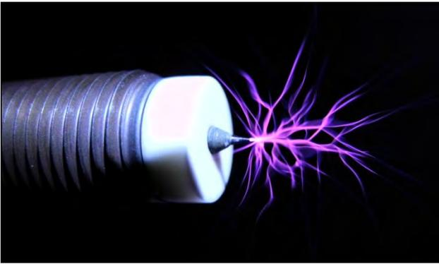
Corona formation on an electrode tip in ambient air
