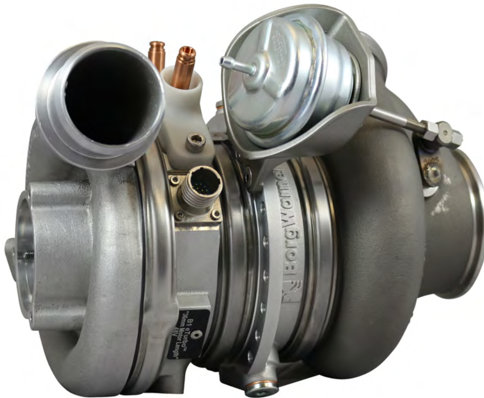
Figure 4. BorgWarner's innovative 48-volt eTurbo™ combines an ultra-high-speed electric motor and turbocharger to provide boost assist or convert exhaust gas flow into electrical energy.
