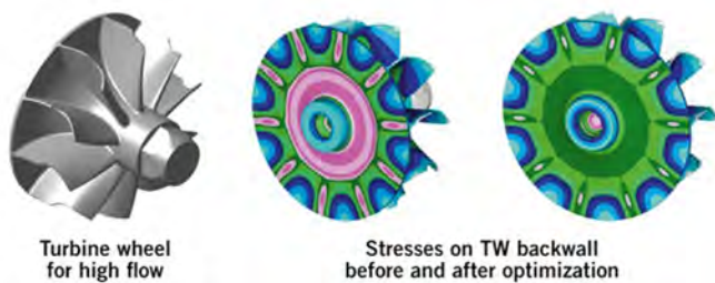
Figure 4. High flow VTG turbine wheel design
