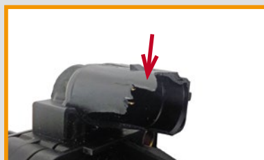
Cracked or damaged plastic parts
