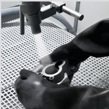
Cleaning and blasting the EGR housing
