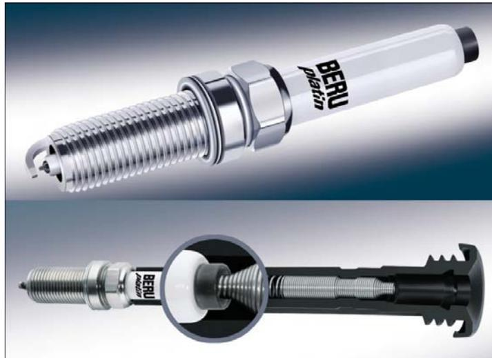
BorgWarner BERU Systems new double platinum spark plugs feature a high-voltage connection specifically designed for today's compact plug top ignition coils. For dependable starts and efficient combustion, the "bowl" contact at the tip of the spark plug's insulator optimizes the connection between the spark plug and plug top ignition coil.
