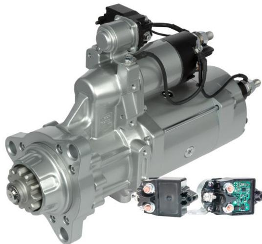
Debuting in the Delco Remy® 39MT™ heavy-duty starter, BorgWarner's new Smart Integrated Magnetic Switch (IMS) protects the starter from six damaging system failures, provides drop-in replacement and offers a more robust warranty than conventional starters.
