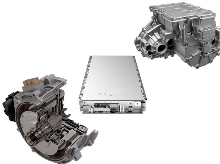
At this year's IAA, BorgWarner demonstrates solutions for hybrid and electric vehicles, such as its P2 module (left), battery packs (middle) and the eAxle iDM (right).
