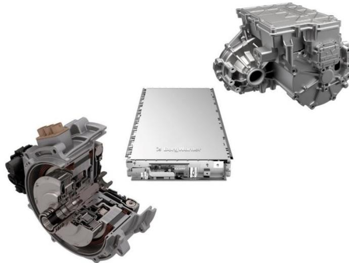
At EV JAPAN 2020, BorgWarner demonstrates solutions for hybrid and electric vehicles, such as its P2 module (left), battery pack (middle) and eAxle iDM (right).
