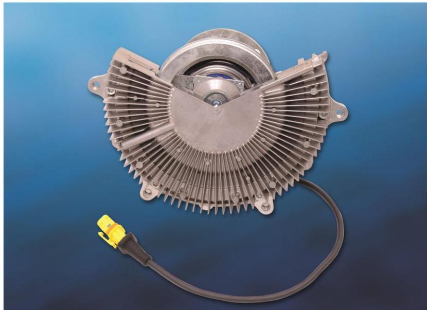
Now produced locally in Brazil, BorgWarner's electronically controlled Viscronic® fan drives respond directly to the engine's cooling needs, precisely controlling the fan speed to deliver efficient engine cooling, improved fuel economy and reduced emissions for trucks, buses and off-highway applications.
