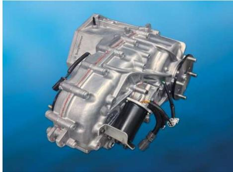
Featuring its proven electronic shift-on-the-fly technology, BorgWarner produces part-time four-wheel drive transfer cases for the 2014 Toyota Tundra pick-up truck.
