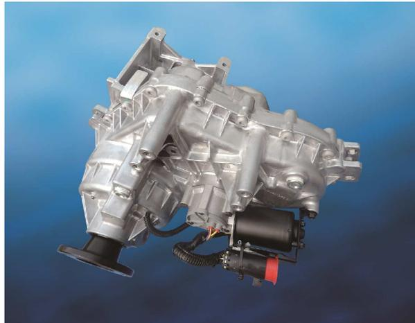
At its manufacturing facility in Beijing, BorgWarner produces numerous all-wheel drive technologies for the Chinese market, including 2-speed Torque-On-Demand<sup>®</sup> transfer cases for the new Sauvana SUV from Foton Motors.
