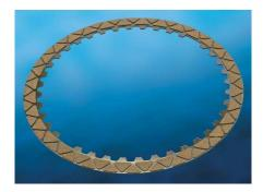
BorgWarner's multi-segment wet friction plate technology for ZF's 8-speed transmission features full-depth grooves between segments of friction material to increase oil flow, improve cooling and prolong clutch life.
